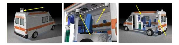
Fig. 3 – Location of video cameras on the mobile platform of MASMED system
