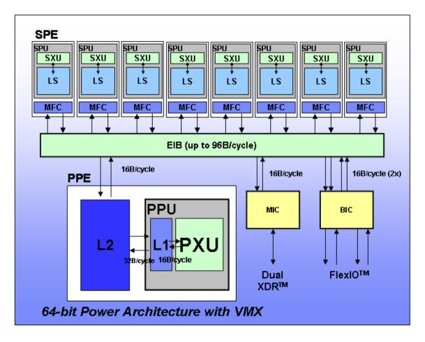
Fig. 6 - The intern architecture of CELL processor used in central system MASMED
