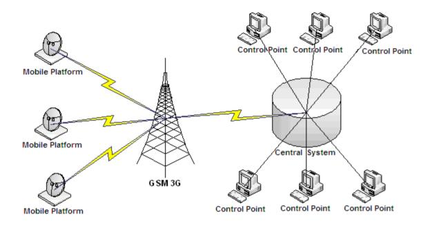
Fig. 1 – The architecture of the MASMED distributed system for collecting, transmission and processing of data streams for the emergency medical system.
